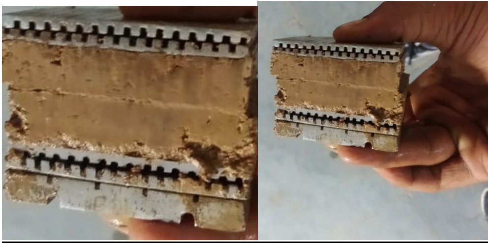
Figure 18 : Shows Direct Shearing of the Soil Sample (samples from the Dump)
