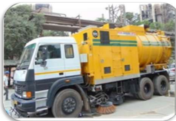
Truck mounted vacuum cum ride-on sweeping machine
