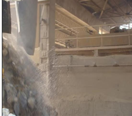
Water spraying System in Crusher Hopper
